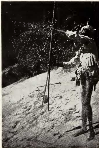
(2) A stone lashed between the jaws of a split bamboo. (After smoothing the edges with a knife.) Very useful in 8 or 10 feet of water to rescue a hook from a boat,
